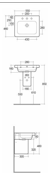
Dimensions: All dimensions in mm. Tolerance of vitreous china & fireclay items:  $\pm$  5% for below 200mm and  $\pm$  3% for above 200mm; for all other items tolerance  $\pm$  1%. Note: Due to a continuing development program to improve design and performance, the manufacturer reserves all rights to vary specifications without prior information. Please note accessories are for photographic use only.
