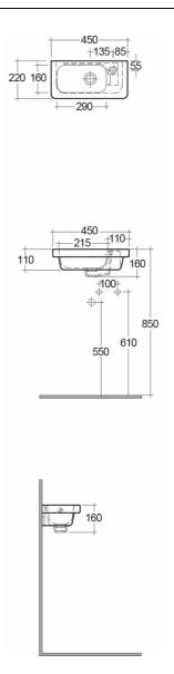
Dimensions: All dimensions in mm. Tolerance of vitreous china & fireclay items: ± 5% for below 200mm and ± 3% for above 200mm; for all other items tolerance ± 1%. Note: Due to a continuing development program to improve design and performance, the manufacturer reserves all rights to vary specifications without prior information. Please note accessories are for photographic use only.
