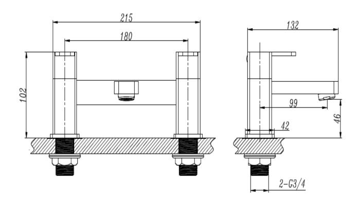
Dimensions: All measurements are in millimeters and are subject to normal manufacturing variations.
