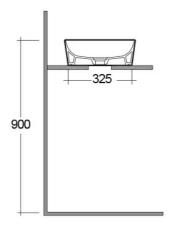
Dimensions: All dimensions in mm tolerance ±5% for below 200mm and ±3% for above 200mm.
